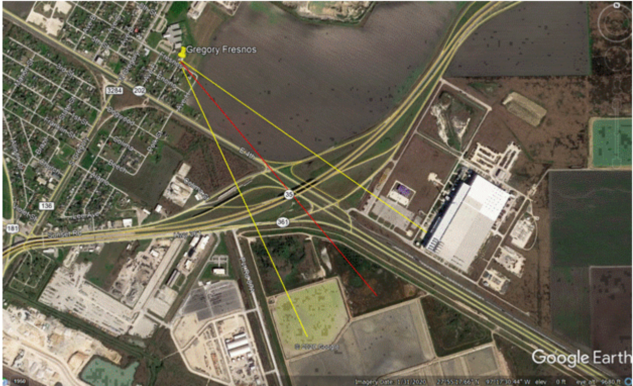
Figure 39. Three 1-mile rays from the Gregory Fresno station, at 140 deg. (center), the most frequent upwind direction and at 125 deg. and 155 deg., which are the easternmost and westernmost directions associated with the peak wind direction in Figure 37
